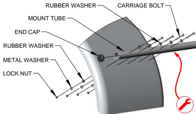
**Tech Tip !!** Use predrilled tube as a drill template
