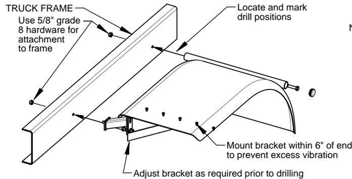
Once mount tubes and brackets are mounted to frame, confirm fender location and drill fender mount holes as required. Depending on mount style, see instructions 3a thru 3j for assembly and hardware details.
